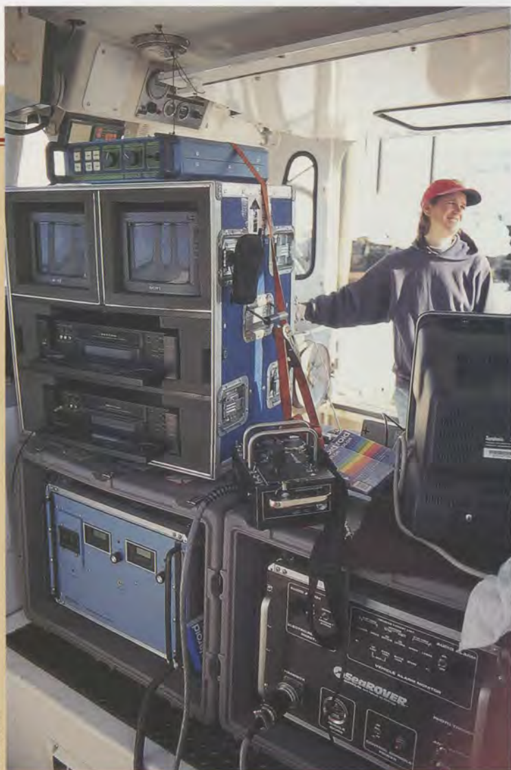
Monitors and other equipment aboard ALICE SIEGMUND record images collected by an underwater side-scanning sonar unit.
